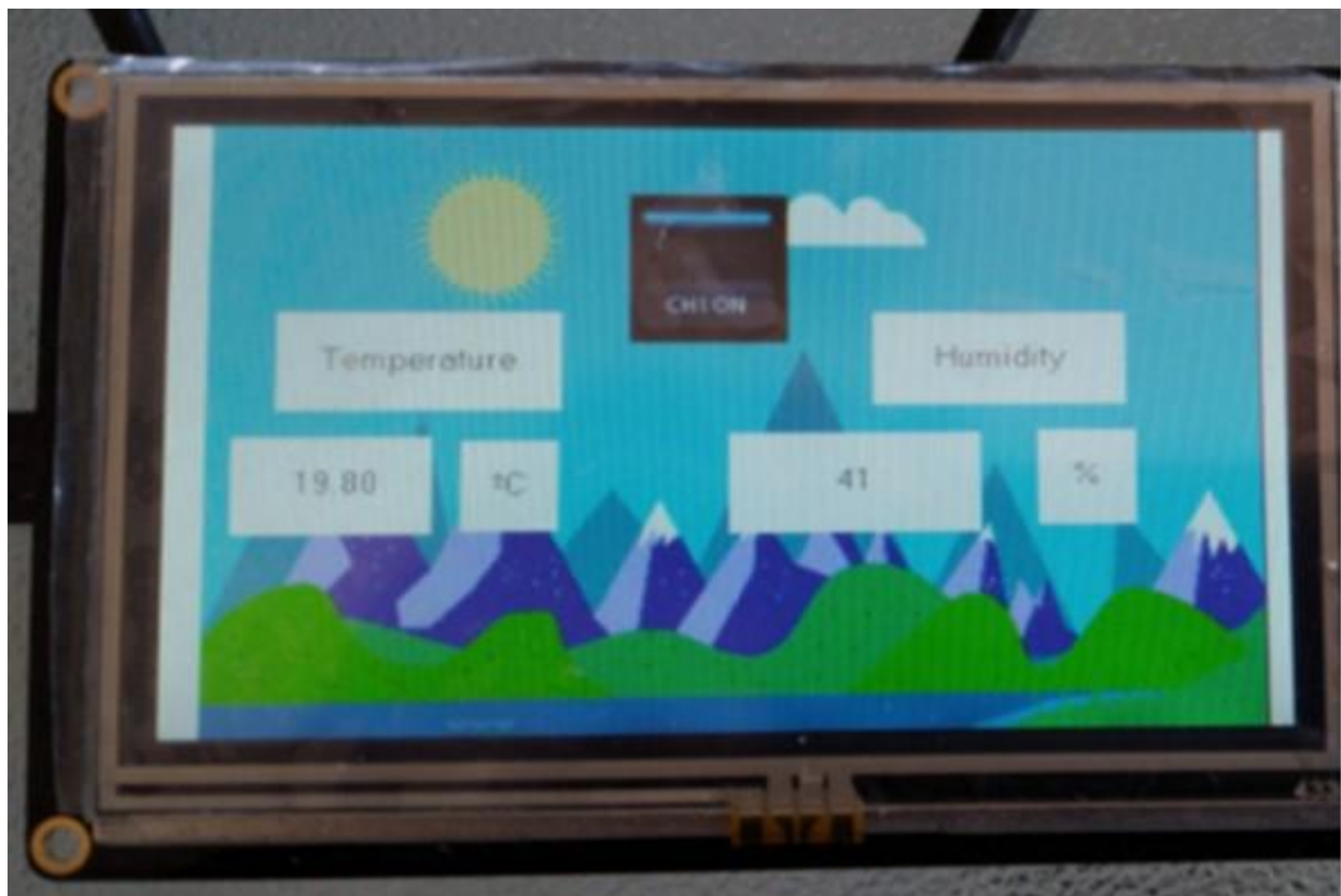
Figure 5.5: Room temperature and humidity analysis in the Control box
